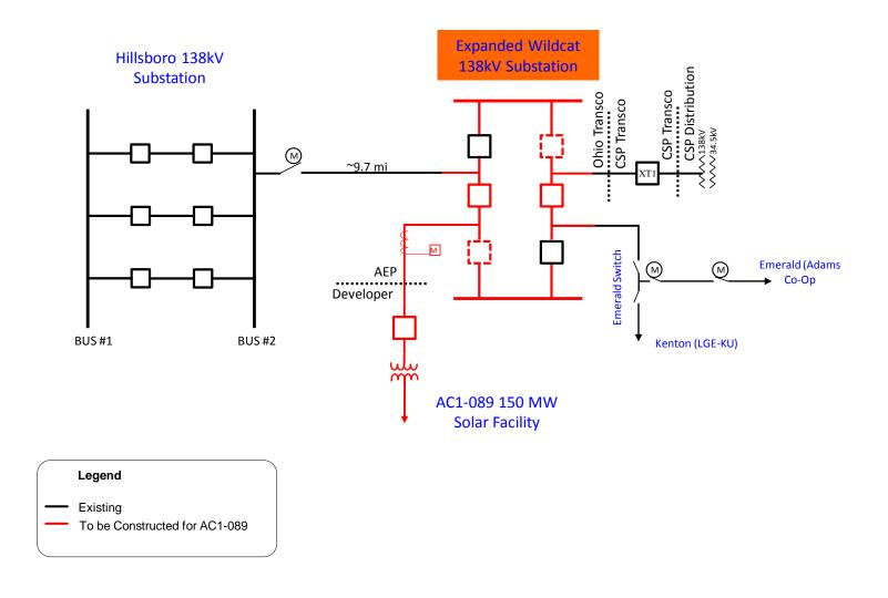
Figure 2: Point of Interconnection (Wildcat 138 kV)
