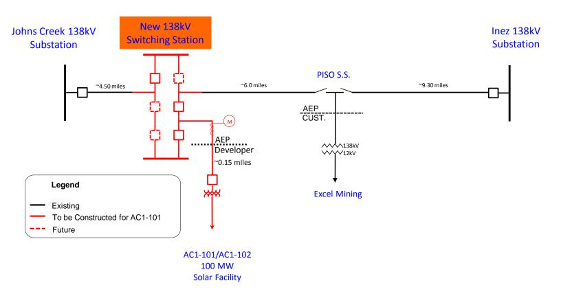
Figure 2: Point of Interconnection (Johns Creek – Excel 138 kV)
