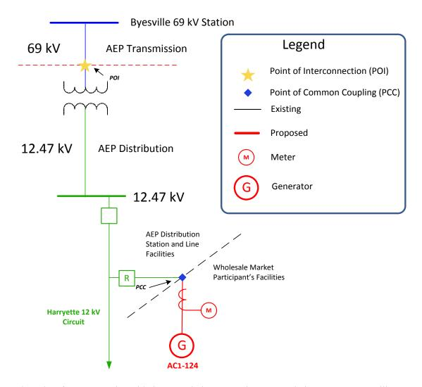
The Point of Interconnection with the transmission system is at Transmission Owner's Byesville 69 kV Station at the Transmission Owner's 69 kV disconnect switch. The point of common coupling (PCC) with the local distribution system will remain at AEP's distribution primary meter facility on the Wholesale Market Participant's premise.
