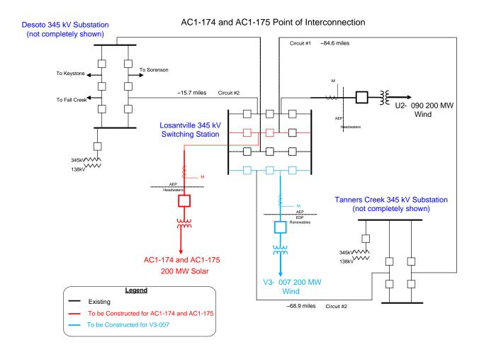
Figure 2: Point of Interconnection (Losantville 345 kV Substation)
