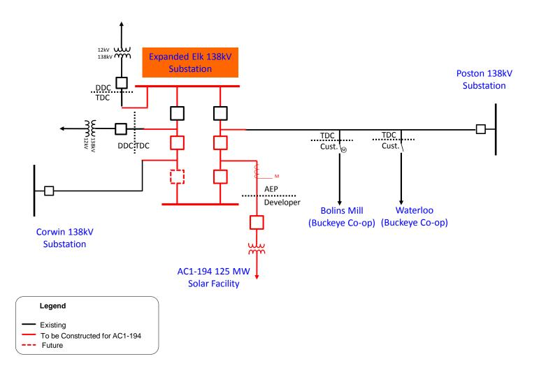
Figure 2: Point of Interconnection (Elk 138 kV Substation)
