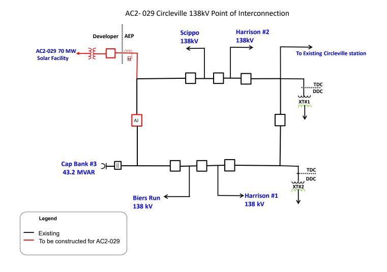
Figure 2: Point of Interconnection (Circleville 138 kV Substation)
