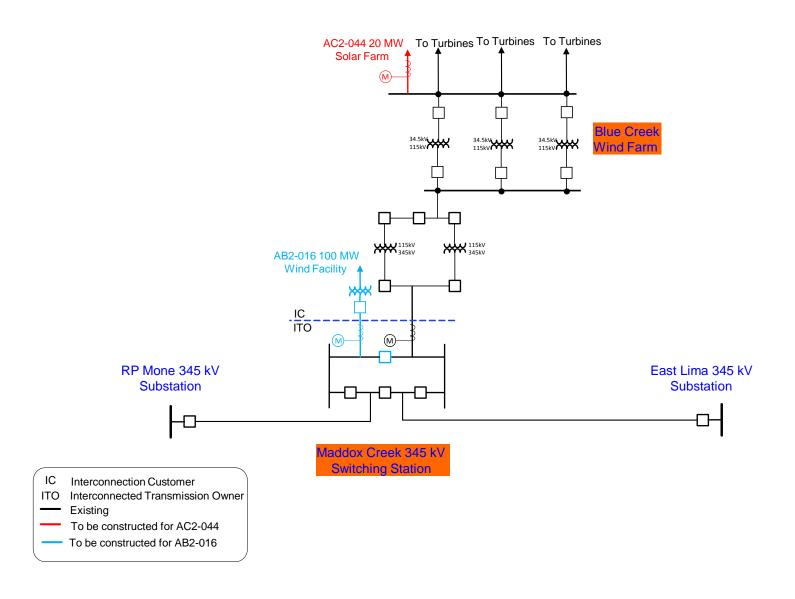
Figure 2: Point of Interconnection (Blue Creek 34.5 kV Collector Station)
