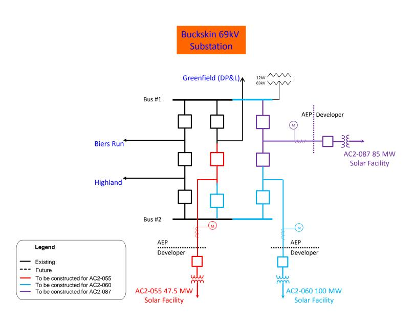
Figure 2: Point of Interconnection (Buckskin 69 kV Substation)
