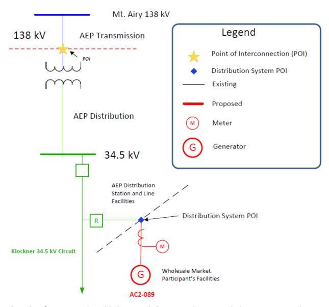
The Point of Interconnection with the transmission system is at Transmission Owner's Mt. Airy 138 kV Station at the Transmission Owner's 138 kV disconnect switch. The point of interconnection with the local distribution system will remain at AEP's distribution primary meter facility on the Wholesale Market Participant's premise.
