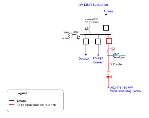
Figure 2: Point of Interconnection (Jay 138 kV Substation)
