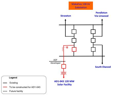
Figure 2: Customer Project Site and Point of Interconnection (Makahoy 138kV Substation)
