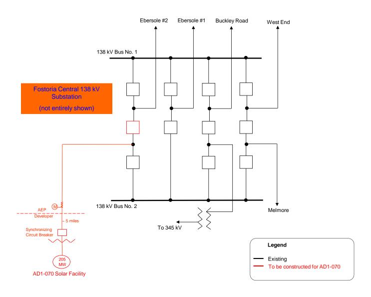
Figure 2: Point of Interconnection (Fostoria Central 138 kV Substation)
