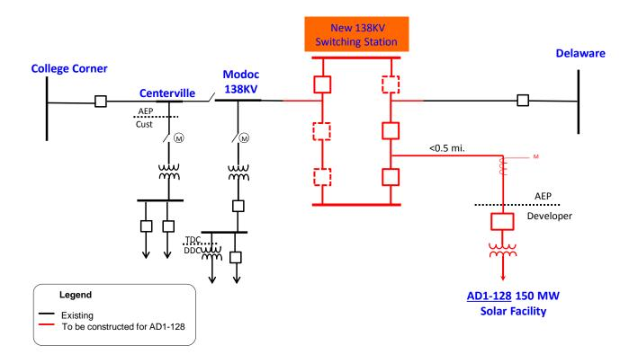
Figure 2: Point of Interconnection (Modoc – Delaware 138 kV)
