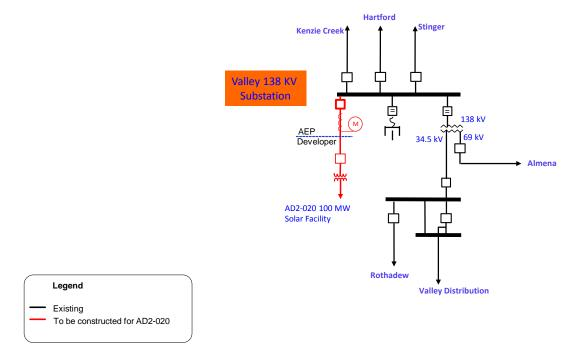
Figure 2: Primary Point of Interconnection (Valley 138 kV)
