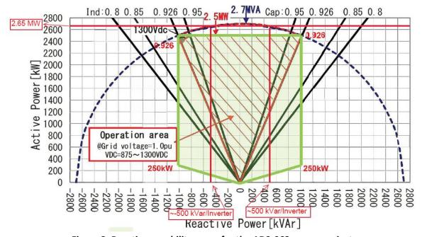
Figure 2: Reactive capability curve for the AD2-062 queue project
