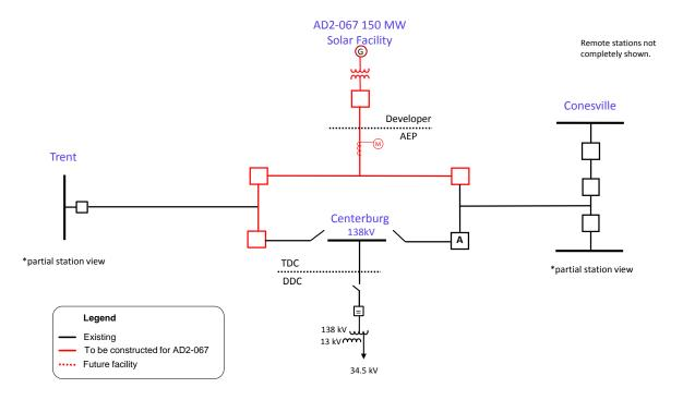
Figure 2: Point of Interconnection (Centerburg 138 kV Substation)
