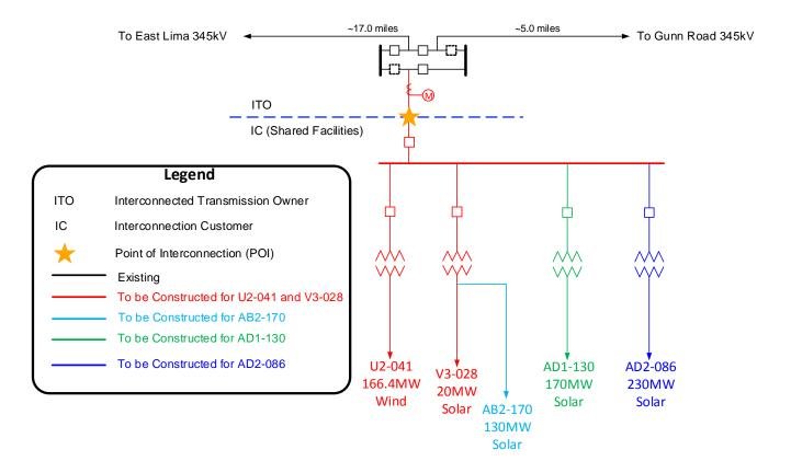
Figure 2: Point of Interconnection (Hardin Switch 345 kV)
