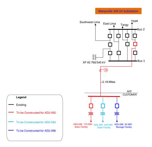
Figure 2: Point of Interconnection (Marysville 345 kV Substation)
