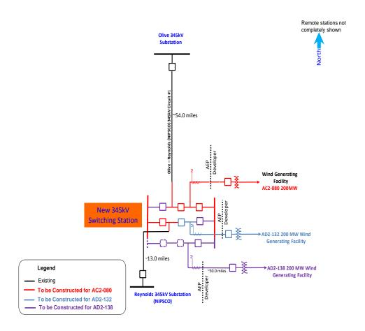
Figure 2: Primary Point of Interconnection (Olive (AEP) – Reynolds (NIPSCO) 345 kV
