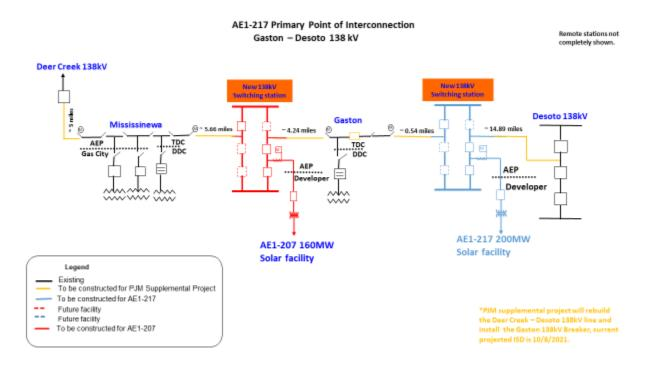
Figure 2: AE1-217 Point of Interconnection (Desoto – Gaston 138kV)
