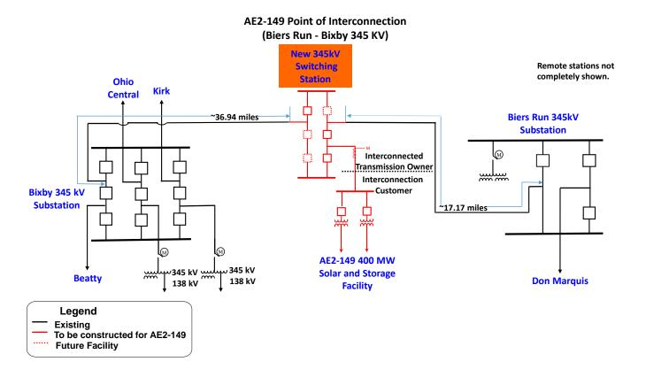
23 Figure 2: AE2-149 Point of Interconnection (Biers Run – Bixby 345 kV)
