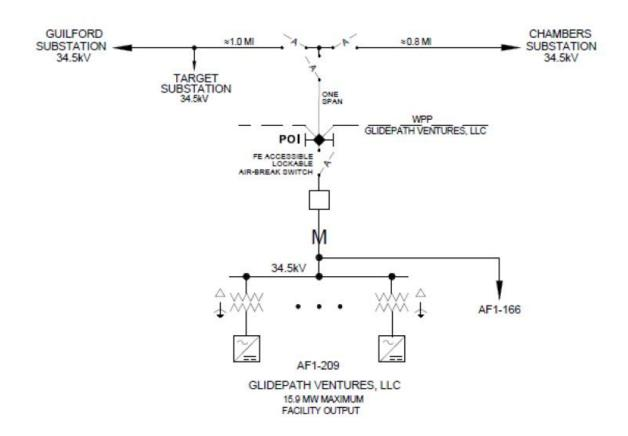
POI (POINT OF INTERCONNECTION) LOCATED AT INTERCONNECTION CUSTOMER'S DEAD-END STRUCTURE WHERE WEST PENN POWER'S (WPP) OWNED 34.5kV TRANSMISSION LINE TERMINATES
