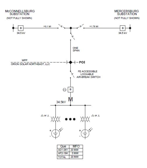
= POI (POINT OF INTERCONNECTION) LOCATED AT ORION SOLAR NORTHEAST, LLC OWNED DEAD-END STRUCTURE, WHERE WEST PENN POWER (WPP) OWNED TRANSMISSION LINE TERMINATES.
