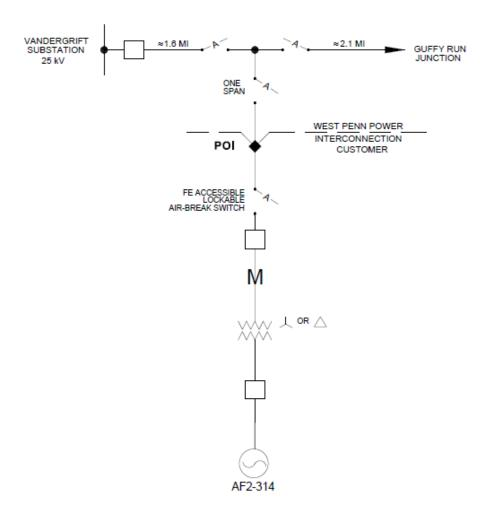
= POI (POINT OF INTERCONNECTION) LOCATED AT WEST PENN POWER OWNED SUBSTATION DEAD-END STRUCTURE WHERE CUSTOMER'S TRANSMISSION LINE TERMINATES
