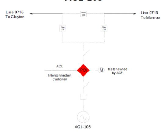
An Interconnection Customer circuit breaker will be required no more than 500 feet from the ACE substation.
