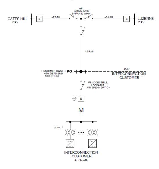
= POI (POINT OF INTERCONNECTION) THE POINT OF INTERCONNECTION IS LOCATED AT THE CUSTOMER OWNED DEAD-END STRUCTURE WHERE WEST PENN POWER (WP) LINE TERMINATES
