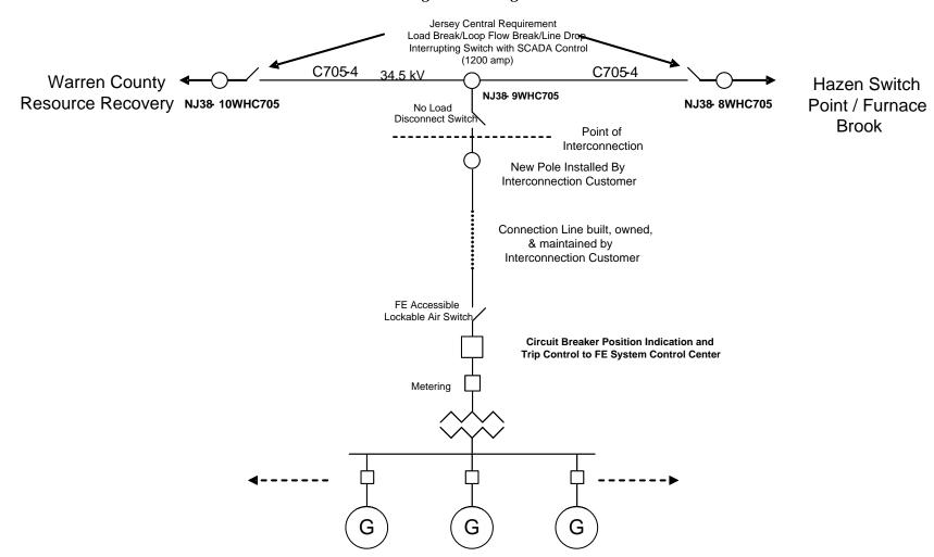
12 MW Total Solar Photo Voltaic Generation
