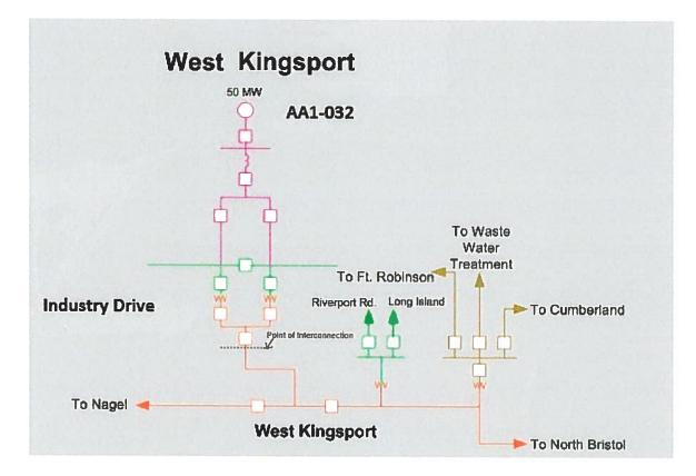
The Point of Interconnection will be at the dead end structure inside the Interconnection Customer's Industry Drive substation with AEP owning the conductors and structures from West Kingsport substation to the dead end structure and the Interconnection Customer owning the dead end structure.
