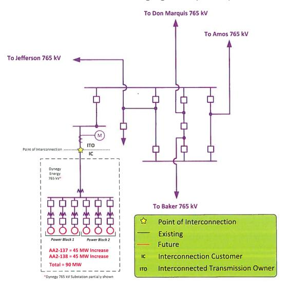
The Point of Interconnection is at the dead end tower in AEP's Hanging Rock 765 kV station with AEP owning the dead end tower and Interconnection Customer owning the conductors and remaining facilities back to the Customer Facility.
