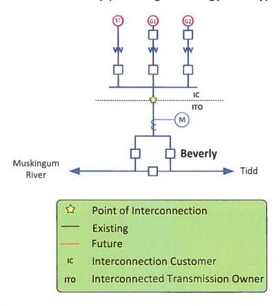
The Point of Interconnection is at the 345 kV disconnect switch in AEP's Beverly substation with AEP owning the disconnect switch, and Interconnection customer owning the conductors connecting to that switch and remaining facilities back to the Customer Facility.
