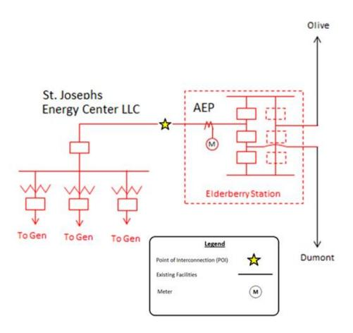
The Point of Interconnection will be the first structure outside of AEP's Elderberry 345 kV station with AEP owning Elderberry station and the first span of conductors required to interconnect the Customer Facility, and the Interconnection Customer owning all structures and remaining conductors to the Interconnection Customer's generation collector station
