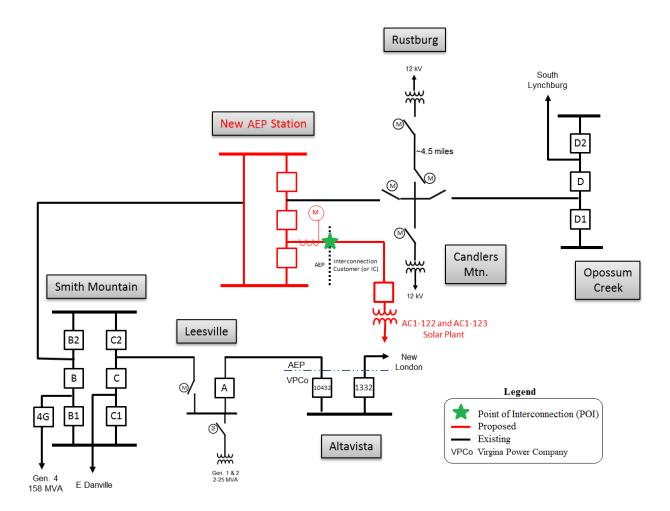
The Point of Interconnection is the structure located inside of the Interconnection Customer's generation collector substation with the Interconnected Transmission Owner owning the span of conductors, including fiber optic cable between the new AEP interconnection substation (the "AC1-122/AC1-123 138kV Interconnection Substation") and the generator collector station, and the Interconnection Customer owning the structure located inside of the generation collector substation.
