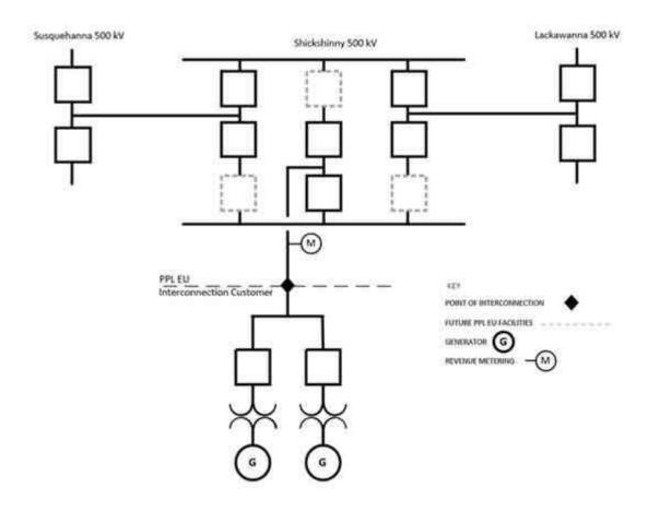
The Point of Interconnection is where the PPL EU 500 kV attachment line terminates (with insulators) onto the dead-end structure in the Interconnection Customer's substation.
