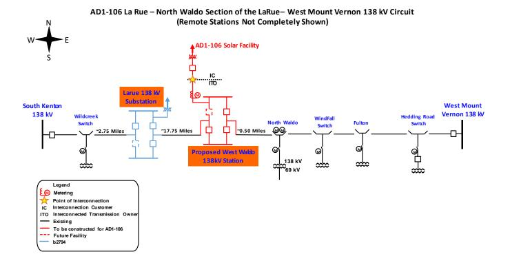
The Point of Interconnection is the first structure outside of AEP's proposed West Waldo 138 kV Substation (such structure being located in Interconnection Customer's collector substation) with the Interconnected Transmission Owner owning the span of conductors, and the Interconnection Customer owning the structure.
