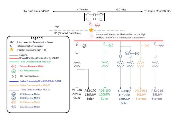
The Point of Interconnection is the first structure outside of AEP's Hardin Switchyard (such structure being located in Interconnection Customer's 34.5-345 kV Collector Substation) with the Interconnected Transmission Owner owning the span of conductors including the optical (fiber) ground wire out of its station, and the Interconnection Customer, and those entities listed in Table 1 of Schedule F under "Associated Interconnection Customer," co-owning the first structure.
