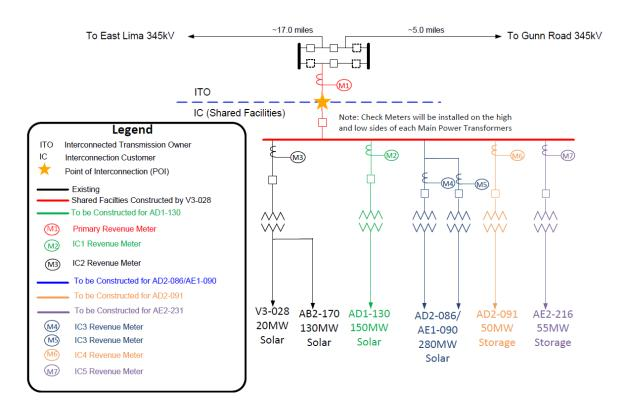
The Point of Interconnection is the first structure outside of AEP's Hardin Switchyard (such structure being located in Interconnection Customer's 34.5-345 kV Collector Substation) with the Interconnected Transmission Owner owning the first span of conductors including the optical (fiber) ground wire out of its station, and the Interconnection Customer and those entities listed in Table 1 of Schedule F under "Associated Interconnection Customer," co-owning the first structure.
