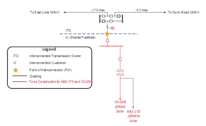
The Point of Interconnection is the first structure outside of AEP's Hardin Switchyard (such structure being located in Interconnection Customer's 34.5-345 kV Collector Substation) with the Interconnected Transmission Owner owning the first span of conductors including the optical (fiber) ground wire out of its station, and the Interconnection Customer owning the first structure.
