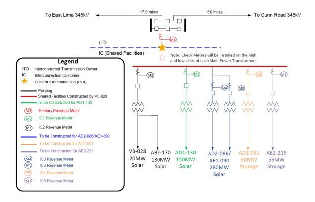
The Point of Interconnection is the first structure outside of AEP's Hardin Switchyard (such structure being located in Interconnection Customer's 34.5-345 kV Collector Substation) with the Interconnected Transmission Owner owning the span of conductors including the optical (fiber) ground wire out of its station, and the Interconnection Customer and those entities listed in Table 1 of Schedule F under "Associated Interconnection Customer," co-owning the first structure.
