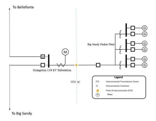
The Point of Interconnection is located inside the Grangston 138 kV switching station with the ITO owning the ridged bus tube before it crosses the station fence into the IC's switching station with the IC owning the flexible jumper wire between the end of the ITO's ridged bus and the start of the IC's ridged bus.
