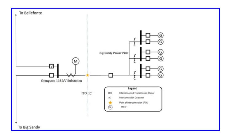
The Point of Interconnection is located inside the Grangston 138 kV switching station with the ITO owning the ridged bus tube before it crosses the station fence into the IC's switching station with the IC owning the flexible jumper wire between the end of the ITO's ridged bus and the start of the IC's ridged bus.
