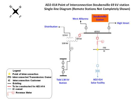
The Point of Interconnection ("POI") is at the first structure in the generator lead line southeast of the Steubenville 69 kV station fence. AEP will own the first span from the Steubenville 69 kV station and the first structure, including the associated jumpers. The Interconnection Customer, will own the opposite span connecting to the POI structure, along with remainder of the 69 kV generator lead line and associated structures back to the AD2-014 generation collector station.
