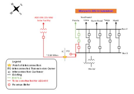
The Point of Interconnection is at the first (dead-end) structure outside of the Marysville 345 kV Station fence. Interconnected Transmission Owner owns the span from the Marysville 345 kV Station to the dead-end, including the jumpers and structure at the dead-end. Interconnection Customer owns the span and structures from the dead-end to the AD2-093 generation collector station.
