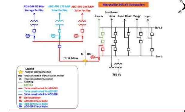
The Point of Interconnection is at the first (dead end) structure outside of the Marysville 345 kV Station fence. Interconnected Transmission Owner owns the span from the Marysville 345 kV Station to the dead-end, including the jumpers and structure at the dead-end. Interconnection Customer owns the span and structures from the dead-end to the AD2-093 generation collector station.
