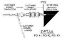
CUSTOMER OWNS CONDUCTOR, INSULATORS, AND IS REQUIRED TO LEAVE ADDITIONAL, JUMPER CONDUCTOR FOR WEST FENN FOWER TO COMMECTTO NEXT DEVICE.
