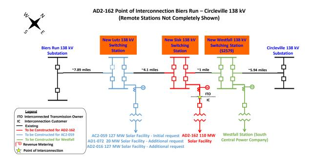
The Point of Interconnection is the first structure outside of AEP's proposed Sisk 138 kV Station (such structure being the station dead-end structure located in the Interconnection Customer's 138 kV collector substation) with the Interconnected Transmission Owner owning the span of conductors from the proposed Sisk 138 kV Station to the Interconnection Customer's dead-end structure, and the Interconnection Customer owning the station dead-end structure and associated jumpers.
