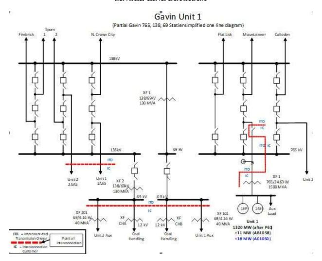
**Gavin Unit No. 1**: Interconnection Customer will own the high voltage lead line connecting Unit No. 1 to the Interconnected Transmission Owner 765 kV switchyard with the Interconnection Customer owning the conductor up to the dead end switch structure located in the Interconnected Transmission Owner 765 kV switchyard.
