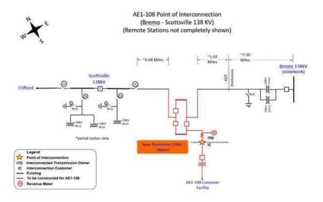
The Point of Interconnection is the first structure outside of AEP's proposed Riverstone 138 kV station (such structure being located in Interconnection Customer's Collector Substation) with the Interconnected Transmission Owner owning the first span of conductors, and the Interconnection Customer owning the first structure.
