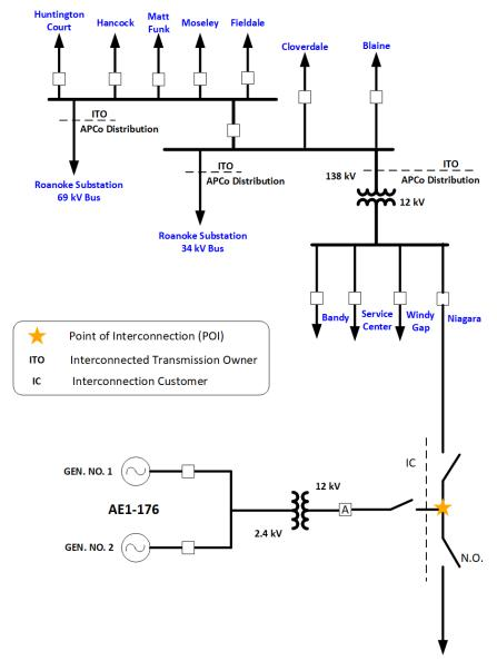
The Point of Interconnection with the local distribution system will remain between the breaker "A" switch and the three terminal tap of Niagara – Vinton 12 kV line.
