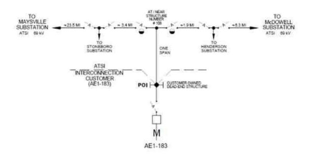
POI (POINT OF INTERCONNECTION) LOCATED AT CUSTOMER OWNED DEAD-END STRUCTURE WHERE ATSI OWNED TRANSMISSION LINE TERMINATES
