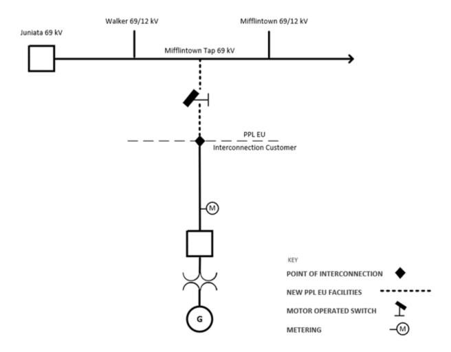
The Point of Interconnection (POI) is where the Interconnection Customer's generator lead line attaches to the PPL EU line tap termination structure.
