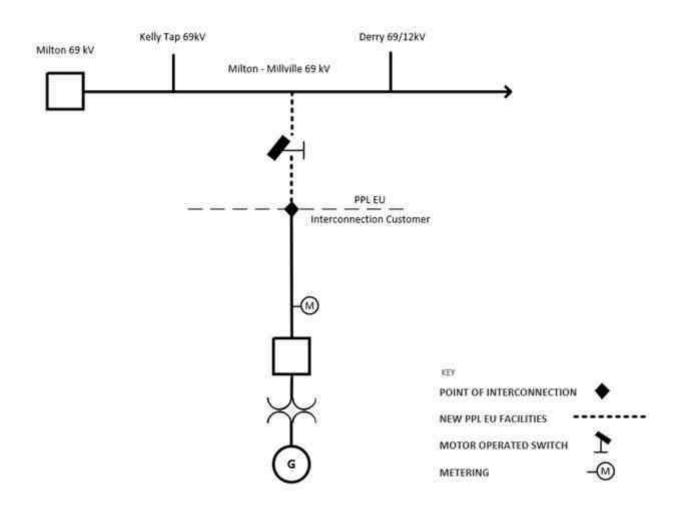
The Point of Interconnection (POI) is where the Interconnection Customer's generator lead line attaches to the PPL EU line tap termination structure. The fiber demarcation is where the Interconnection Customer fiber terminates in the PPL EU fiber splice box on the termination structure.
