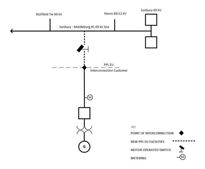
The Point of Interconnection (POI) is where the IC generator lead line attaches to the PPL EU line tap termination structure. The fiber demarcation is where the IC fiber terminates in the PPL EU fiber splice box on the termination structure.
