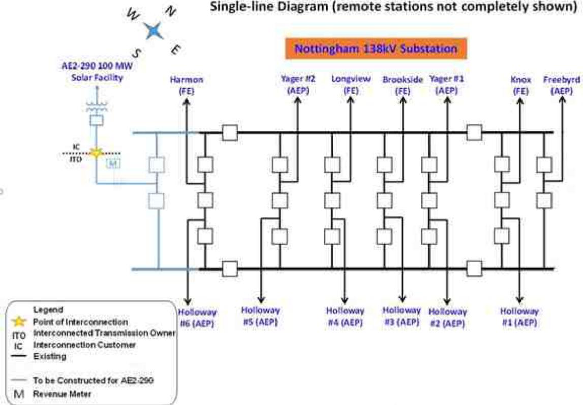
The Point of Interconnection is at the first (dead-end) structure outside (north-west) of the Nottingham 138 kV Station fence. Interconnected Transmission Owner owns the span from the Nottingham 138 kV Station to the dead-end, including the jumpers and structure at the dead-end. Interconnection Customer owns the span and structures from the dead-end to the AE2-290 generation collector station.
