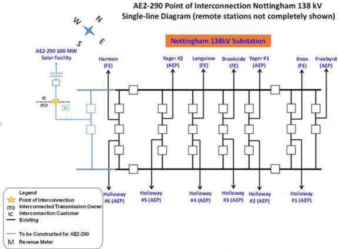
The Point of Interconnection is at the first (dead-end) structure outside (north-west) of the Nottingham 138 kV Station fence. Interconnected Transmission Owner owns the span from the Nottingham 138 kV Station to the dead-end, including the jumpers and structure at the dead-end. Interconnection Customer owns the span and structures from the dead-end to the AE2-290 generation collector station.
