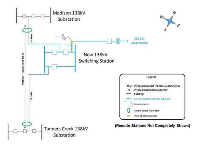
The Point of Interconnection is at the first structure outside of AEP's new 138 kV switching station (such structure being the dead-end structure located in Interconnection Customer's 34.5-138 kV Collector Substation) with the Interconnected Transmission Owner owning the span of conductors to the dead-end structure, and the Interconnection Customer owning the dead-end structure.
