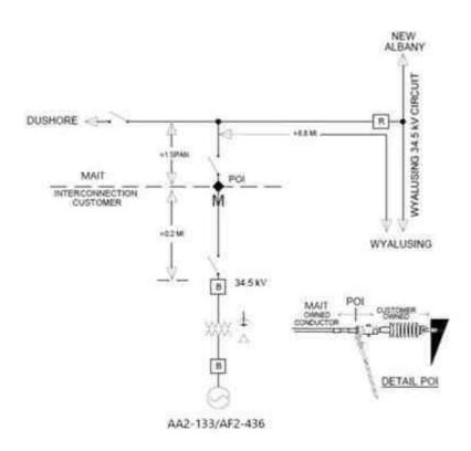
POX POINT OF INTERCONNECTION, LOCATED AT OUSTOMER OWNED DEAD-END STRUCTURE
