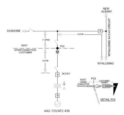
POI (POINT OF INTERCONNECTION) LOCATED AT CUSTOMER OWNED DEAD-END STRUCTURE
